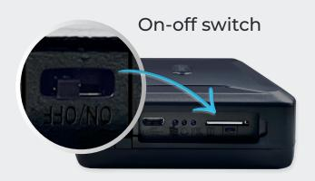
When activation is successful, turn on the GPS tracker by sliding the switch located under the protective rubber to the right. The LED lights then activate. To switch off, move the switch to the left.
