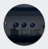
**Is the red LED on?** The GPS tracker is charging. **Is the red LED off?** The GPS tracker is fully charged (please note that this may not be the case after the first charge).
