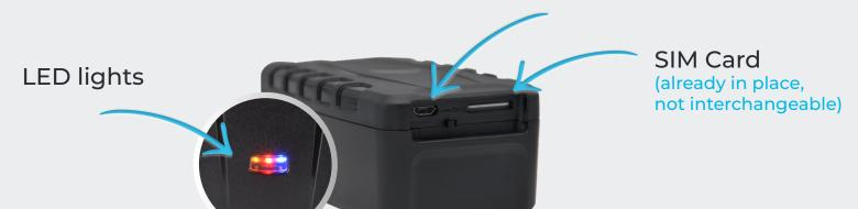
Before using it for the first time, you should charge the GPS tracker for about 8-12 hours. Connect the supplied charging cable to the charging port on the GPS tracker. Then attach the USB port to the power socket adapter. Once the GPS tracker is connected to the power source, please charge it until the red LED turns off.
