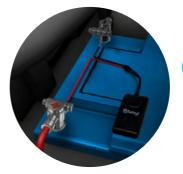
Connect the tracker to the battery. Connect the red cable with the fuse to PLUS (+). Connect the black cable to Minus (-).
