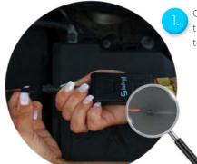
Connect the tracker via the black plug function to the wiring harness.
